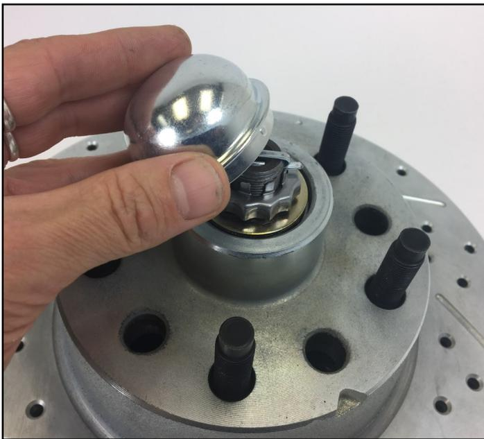
**7.** Now install the dust cap. Be careful not to dent the dome portion which may lead to interference with the cotter pin.
