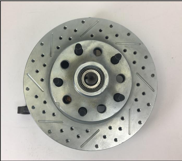
**5.** Next install the correct side rotor. Be careful not to damage the wheel seal when going over the base of the spindle pin. Thread the spindle nut on and snug. (Right side/passenger shown)
