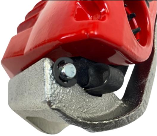
**INSTALL THE E-CLIP INTO THE GROOVE ON THE END OF THE PIN STICKING THROUGH THE FRONT OF THE CALIPER AS SHOWN TO SECURE THE ANCHOR TO THE PADS. REPEAT THIS PROCESS FOR THE OTHER CALIPER.**
