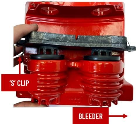
**INSERT THE PAD INTO THE PISTONS AS SHOWN. THE 'S' CLIP INSTALLED PREVIOUSLY, SHOULD BE OPPOSITE THE BLEEDER. INSTALL THE OUTSIDE PAD WITH THE 'S' CLIP OPPOSITE THE BLEEDER.**
