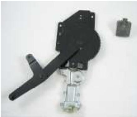
The Nu-Crank Switch will be mounted directly to the regulator.
