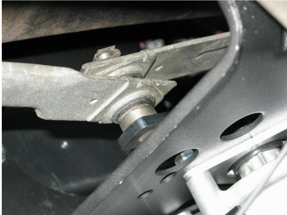
Figure 8 - Attach Wiper Linkage to Pitman Arm
