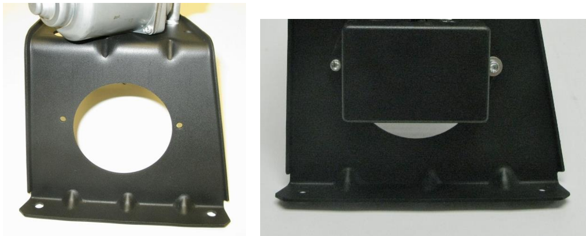
Figure 7 – Mount the Wiper Control Module
