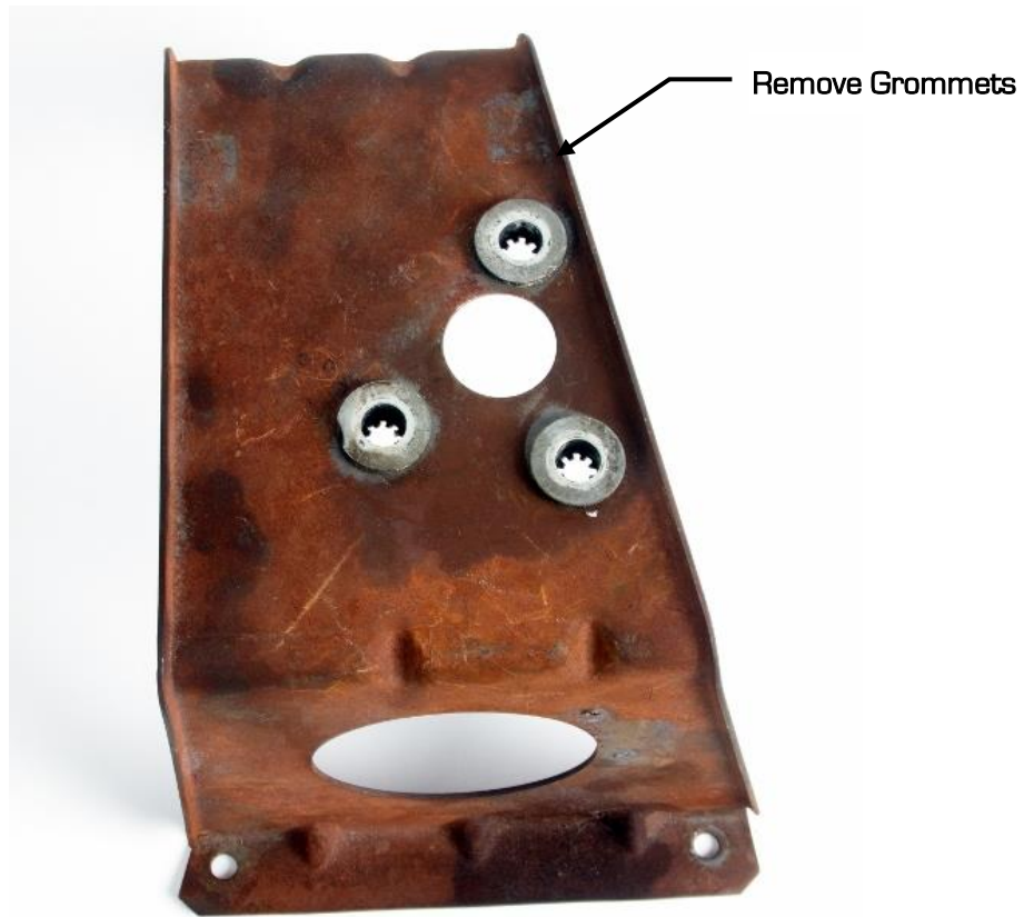
Figure 2 - Factory Wiper Motor Mounting Bracket
